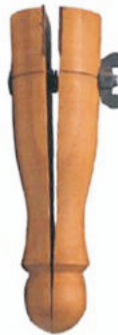
TM-5117 Wood Ring Clamp Used for holding and securing rings in various positions while being worked upon. The ring clamp is a handy tool for holding rings to be filed, drilled or polished. Made from wood, this clamp holds the ring vertically between two leather pads. The pads are tightened and released from around the ring by turning the wing nut on the side of the clamp. Makes jobs such as soldering easy
