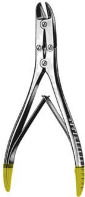
JT-21-1009: Pin Cutting Pliers, Multiple Action, 4-screws, for soft pin up to 2.00 mm and hard pin up to 1.5 mm dia. Size 7" also available in 7 ½" 8", 8 ½" 9" and 9 ½" with TUNGSTEN CARBIDE (TC) Tip, Gold plated handle, LIFE TIME GUARANTEE
