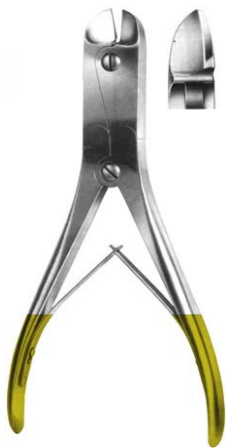
JT-21-1011: Pin Cutting Pliers Multiple Action, 4-screws Front cutting action for soft pin up to 3.5 mm and hard pin 2.5 mm, dia Size 9" also available in 7", 7 ½" 8", 8 ½" 9 1/2" and with TUNGSTEN CARBIDE (TC) Tip, Gold plated handle, LIFE TIME GUARANTEE
