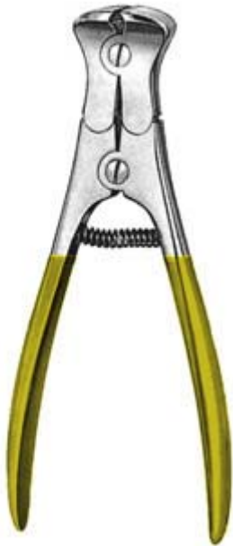
JT-21-1014: Pin Cutting Pliers Multiple Action, 4-screws Lateral cutting action for soft pin up to 2.5 mm and hard pin 2.0 mm, dia Size 7" also available in 7 ½" 8", 8 ½" 9" and 9 ½" with TUNGSTEN CARBIDE (TC) Tip, Gold plated handle, LIFE TIME GUARANTEE
